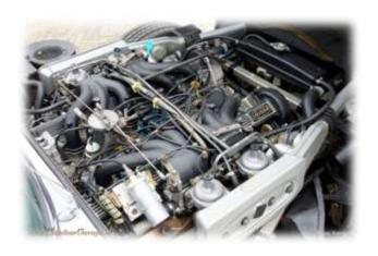
This all new alloy V-12 was only 80 lbs heavier than the 6 cylinder engine it replaced. It was also the first mass-produced V-12 since the late-30's Lincoln engine. Jaguar's V-12 engines had some bad P.R. problems but it turns out that most of the issues were due from lack of proper maintenance from the owners. If the engines were kept cool and fluids changed regularly the engines were dependable.
