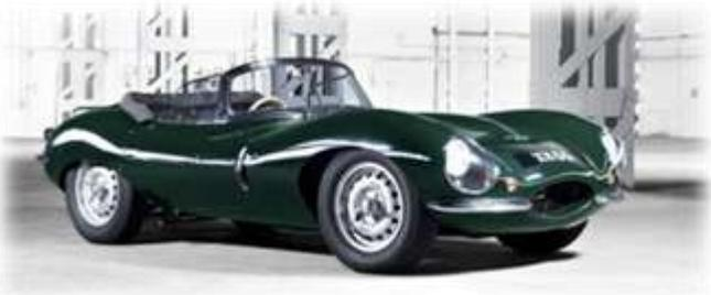
Hannig said Jaguar took a three-dimensional scan of the surviving XKSS that most closely resembles the original production version and will compare it to design blueprints to replicate the car. It will be built by hand.
