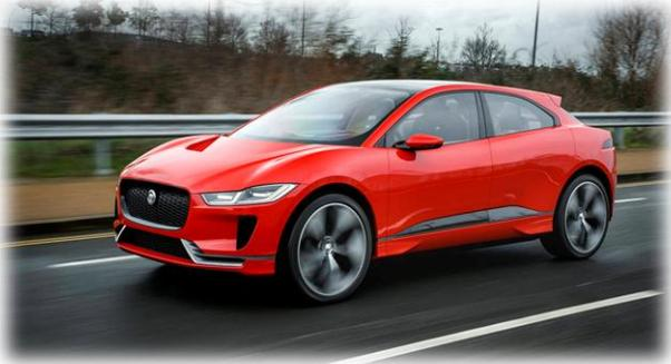
The I-Pace concept has electric motors in the front and rear axles with a combined output of 400 hp and 516 lb-ft of torque, which will allow it to get from 0-60 mph in just 4.0 seconds if you're in a hurry. The compact SUV/hatch is powered by a 90-kWh lithium-ion battery, and Jaguar expects it to have an EPA-estimated range of 220 miles on a full charge; an 80 percent charge is said to take just 90 minutes, with a full recharge in just two hours when a 50-kW DC fast-charging terminal is used.
