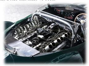
Soon switching to mechanical fuel injection and running as an integral, structural part of the XJ13's chassis, the complex, 503 HP V12 and its 5-speed ZF transaxle acted as the sole support structure aft of the rear bulkhead, to which suspension was directly mounted.
